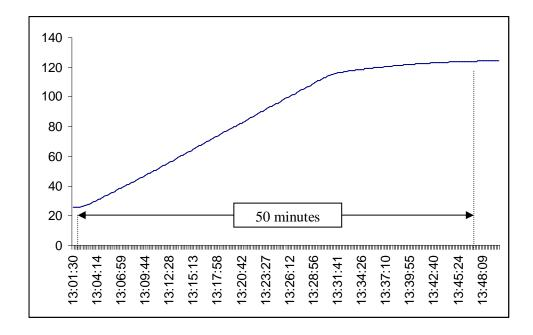
The above graph shows the warm up time of the Orion M to 125°C, the liquid medium is Isotech C10 oil.
