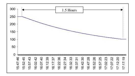
The above graph shows the cooling coil in use for the Orion H. The graph show a cool down time from 250°C to 100°C in a time of 90 minutes. The cooling medium was water under tap pressure. The liquid medium was Isotech VH oil.
