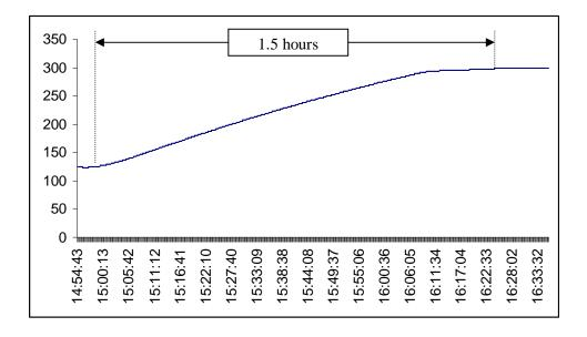
The above graph shows the warm up time of the Orion H from 125°C to 300°C. The liquid medium is Isotech VH oil.
