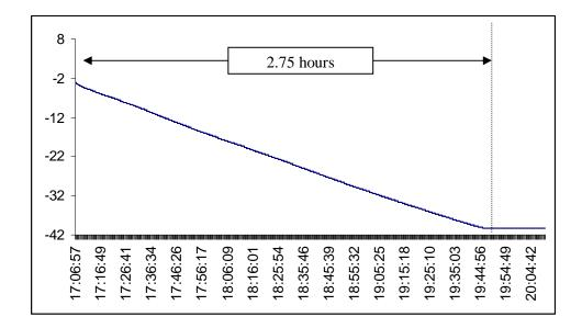
The above graph shows the typical cool down data for the Orion M. The liquid medium was Methanol and the setpoint - $40^{\circ}$ C.
