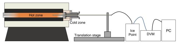
Figure 1 NPL's homogeneity scanner and peripheral equipment.
