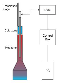
Figure 2 Isotech Homogeneity Scanner and peripheral equipment.
