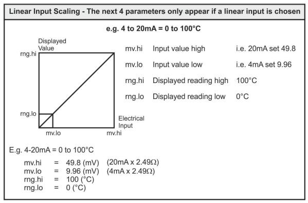
**EXAMPLE:** From the input menu iP set the mv.hi, mv.lo, rng.hi and rng.lo parameters to suit see table below:
