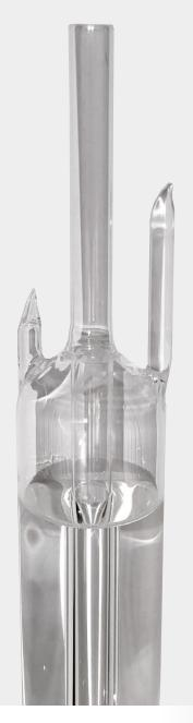
The Isotech-Jarrett cells have been in production since 1958. An independent comparison showed the first cell to be within 0.000006°C of the reference cell. The most recent international study organized by BIPM consistently shows labs using both recent and older Isotech-Jarrett cells tightly grouped, tens of  $\mu$ K around the BIPM reference value.
