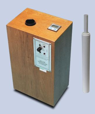
Second only to the Water Triple Point and in many ways, because of its ease of use and purity, superior to it, is the Gallium Melt Point. At 29.7646°C this is a very convenient temperature.
