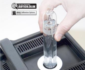
Isotech Liquid Baths and Dry Blocks have options to maintain water triple point cells
