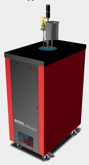
The Isotech Argon Triple Point Apparatus is a robust, simple to use and affordable solution for the realisation of the argon triple point.
