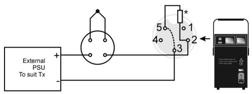
\*2.49Ω resistor fitted internally (Pins 2 and 5). Link Pins 3 and 5 for transmitter inputs. Remove link for T/C's and PRT's. Socket Pins shown from Panel View
