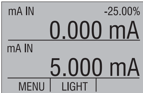
Figure 6. Measuring mA with Input/Output Terminals
